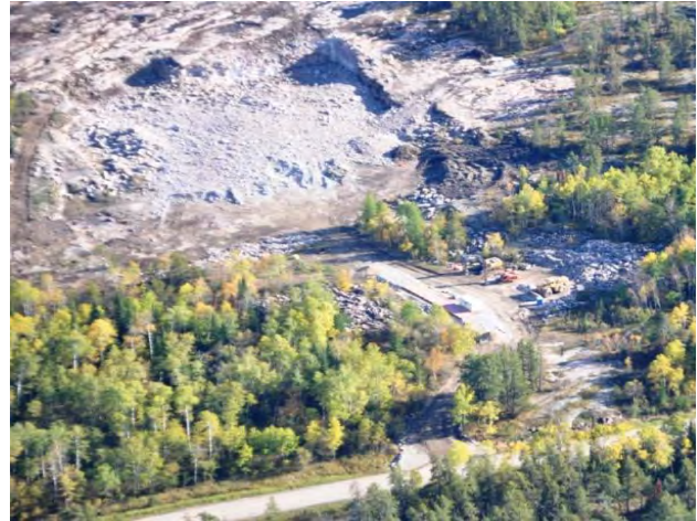
Photo 2: A borrow pit next to a highway with a vegetative berm to shield the area from view.
