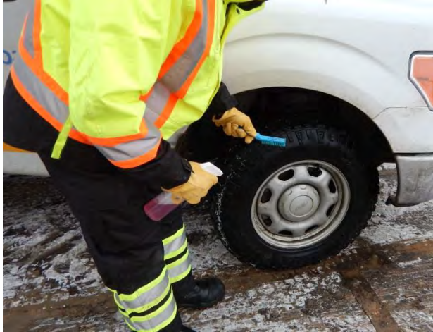
Photo 5: Truck tires are scrubbed clean of any soil or debris before driving on to the next site.
