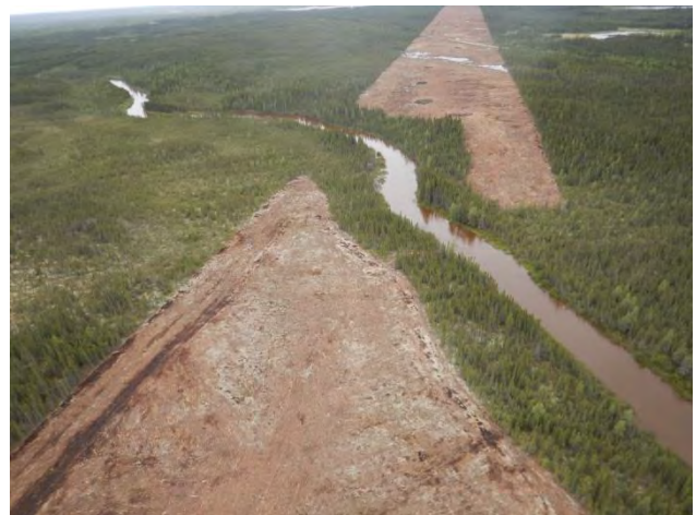
Photo 6: A 30 m riparian buffer established from the ordinary high water mark.
